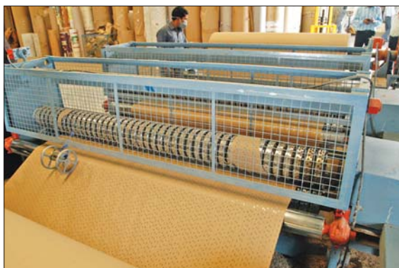
The indigenously made perforating machine is the fastest in the world claims Krishna Lamicoat
